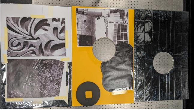
Fig. 5. Example of textures used for physical data augmentation for training. Multiple panels have been created to be affixed around the mock-up satellite’s docking port or to fully replace the mock-up.
